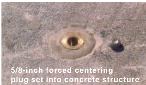
Figure 2-9. Target plug set on concrete structure. Forced centering device on tribrach shown upside down
